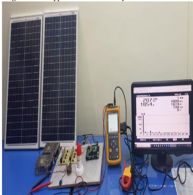
Figure.6 Prototype Hardware of PV system based CHB MLI
