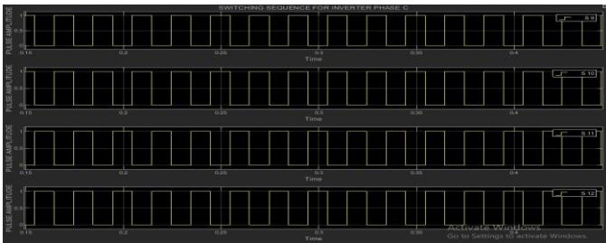
Figure 10 Switching Sequence of Inverter Phase C
