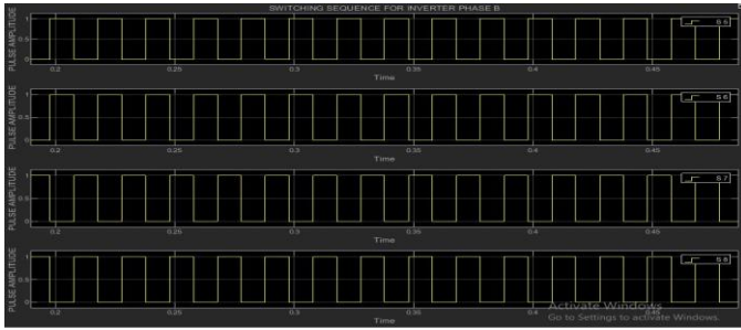
Figure 9 Switching Sequence of Inverter Phase B
