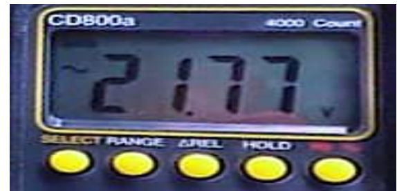
Fig:17b voltage across heavily loaded transmission line
